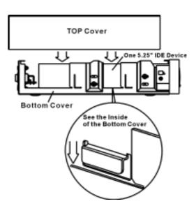
b) Slide the top cover forward until it fits tight within the front groove guide.
